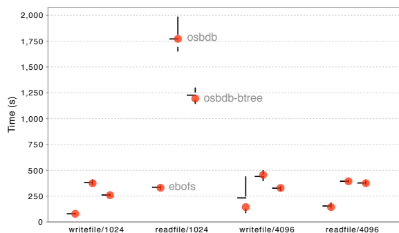
Figure 4: readfile and writefile, operating on a 1GiB file in 1KiB and 4KiB chunks. The above represents sixteen runs of the workload.
